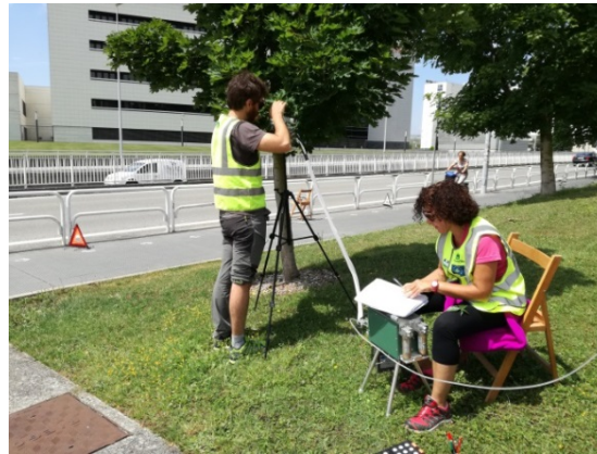
Figure B4.1 Measurement campaign of stomatal conductance in urban vegetation
