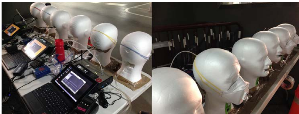
View of the prototypes used to perform the quality control of anti-pollution facemasks
