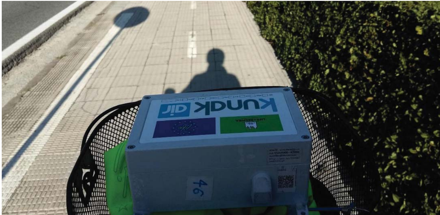
Figure 1. Cycling on a bike path with the analyser in its usual position - in the basket.
