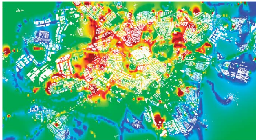
Figure 11. Concentration of CO. The highest levels (indicated in red) correspond to the stagnant areas next to the NW slope of the city, while suburban neighbourhoods have lower concentrations (indicated in blue).
