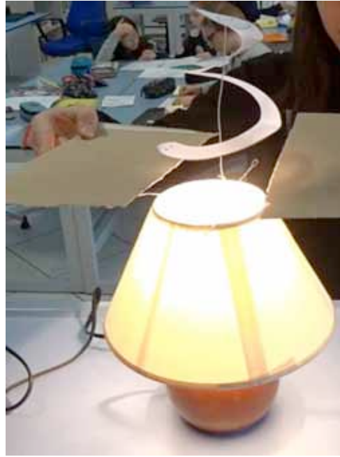
Figure 2. Paper spiral spinning at a speed varying with the wattage of the bulb
