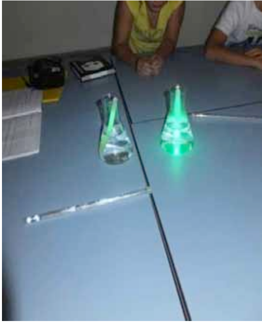
Figure 1. Glow sticks in water emitting different light intensities at different temperatures
